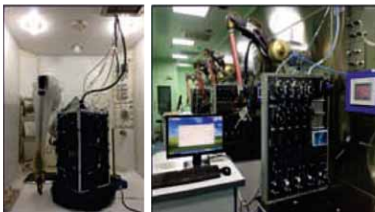
Fig. 10: Thallium Chemistry hot cell with Tl-chemistry module
