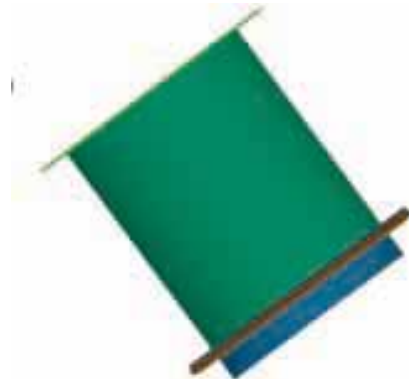
Fig. 4(c): Inverted corner drop of MTP-1200 cask
