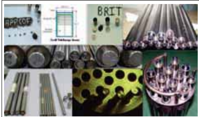
Fig. 2: Sealed sources: Cobalt-60 Teletherapy Sources (CTS), W-91 and BC-188 model Multi-Purpose Gamma Irradiator Sources
