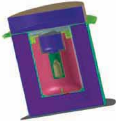
Fig. 2(a): Volume-cut view of MTP-1200 cask
